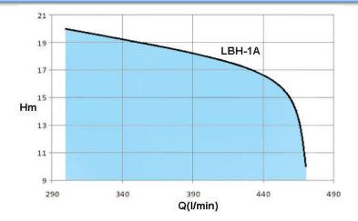
Motor Body: Cast IronMotor power: 2 HPMax. flow rate: 470 I/minDynamic head up to: 20 mThree phase: 415V -15% & +6 %2 - pole submersible motor50Hz (n = 2880 RPM)
