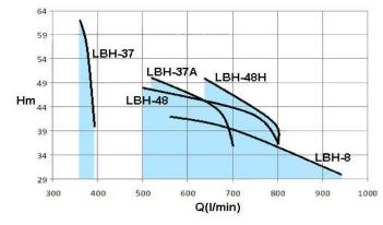
**Motor Body** : Cast Iron : 7.5 HP Motor power Max. flow rate : 1660l/min Dynamic head up to : 62 m
